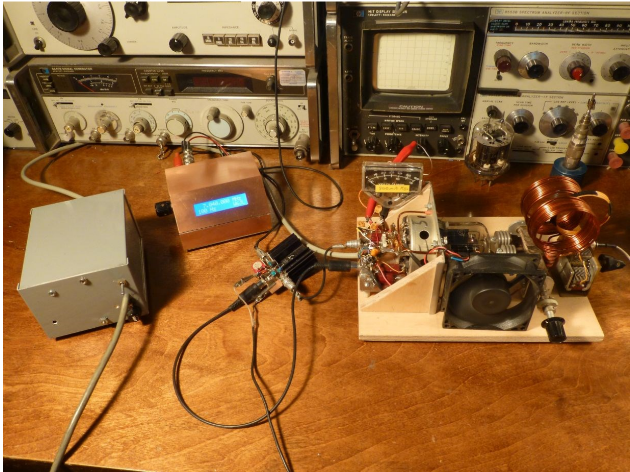
Complete transmitter with (L-R) power supply, VFO, driver, and 829B amplifier.
